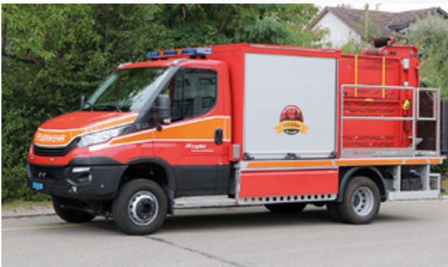
Payload: e.g. 2,000 m B-hose or 1,000 m A-hose
