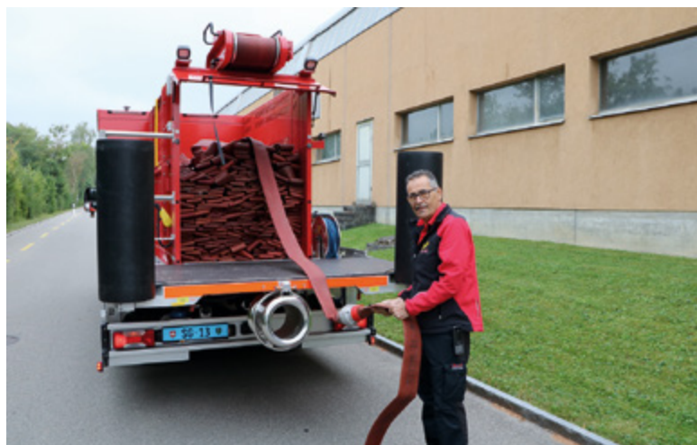
Brändle's senior technical expert Fredy Röthenmund is considered to be the developer of the Brändle hose laying system. The hose box and the stainless steel recovery chute at the rear are clearly visible.
