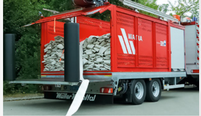
Payload: e.g. 6,000 m B-hose or 3,500 m A-hose
