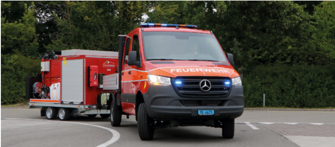
The hose laying system used by the Matzingen-Stettfurt fire brigade on a 3.5 t Brühlmann trailer. The multi-purpose vehicle mounted on an MB Sprinter 319 CDI 4 × 4 was also delivered by Brändle in 2020. (Photos: J. Thorns)
