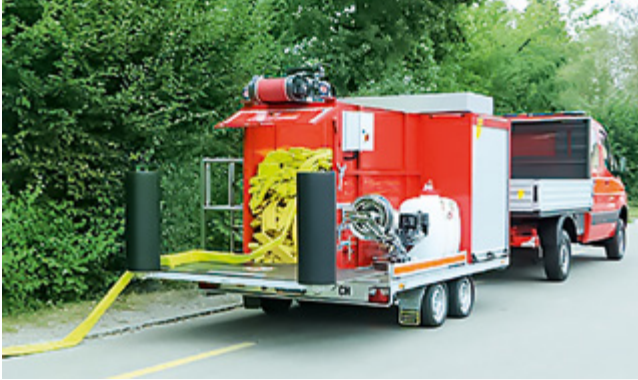
Payload: e.g. 2,400 m B-hose or 1,500 m A-hose
