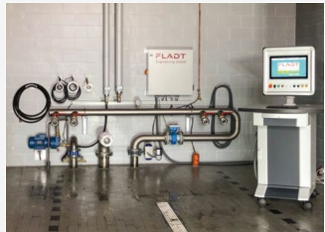
View inside pump test room with ideal connection options for suction and pressure hoses
